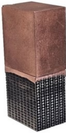
Figure 8 W lattice infiltrated with Cu, then diffusion bonded to CuCrZr
