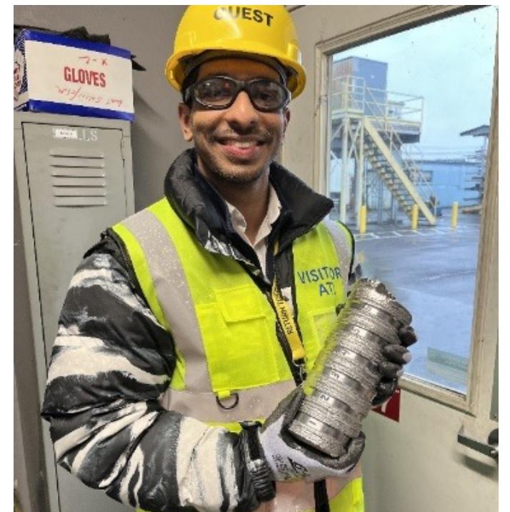
Figure 34 Lead Fusion Technologist, Davidson Sabu pictured with a plasma arc melted V44 ingot, ready for rolling into plate in ATI’s Pittsburgh facility
