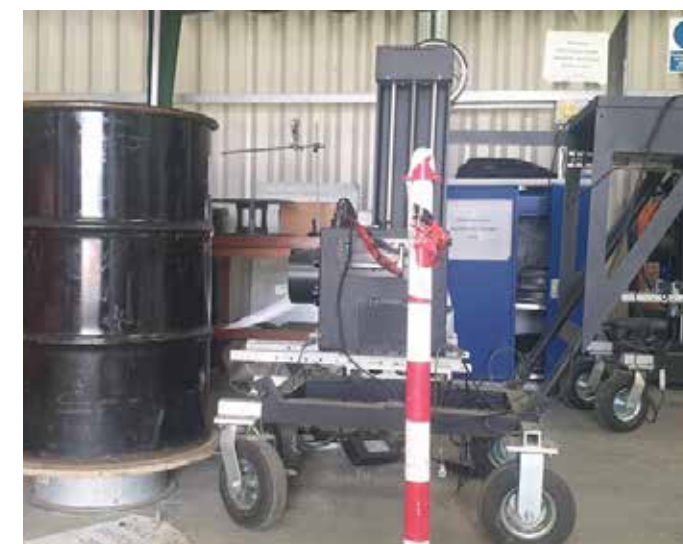
Figure 37 Drums were manually sorted and scanned using state-of-the-art high-purity germanium detectors
