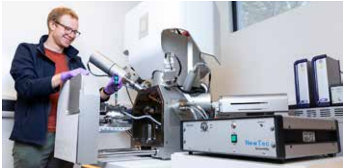
Figure 36 is In-situ mechanic testing stage used to evaluate fundamental modes of deformation
