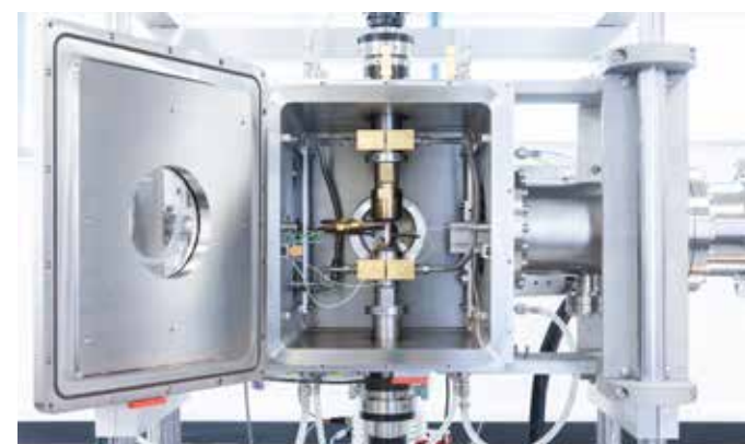
Figure 31 ZWICK Cappa vacuum furnace inside the AMT lab
