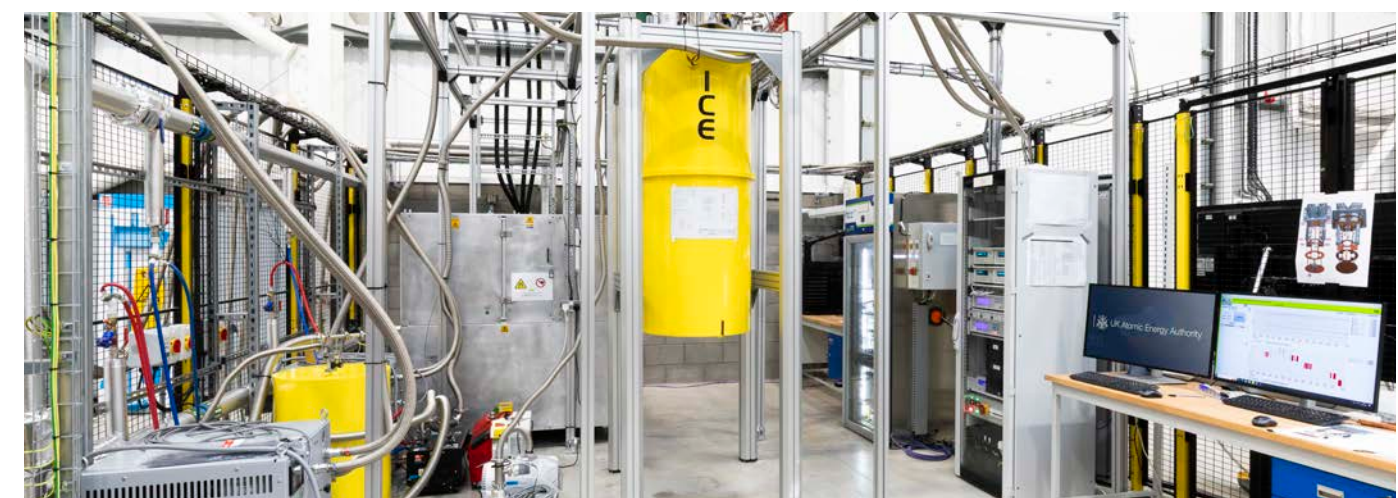
ELSA is a wide-bore superconducting magnet system that will be used to test and develop magnet component designs for STEP and other projects.
