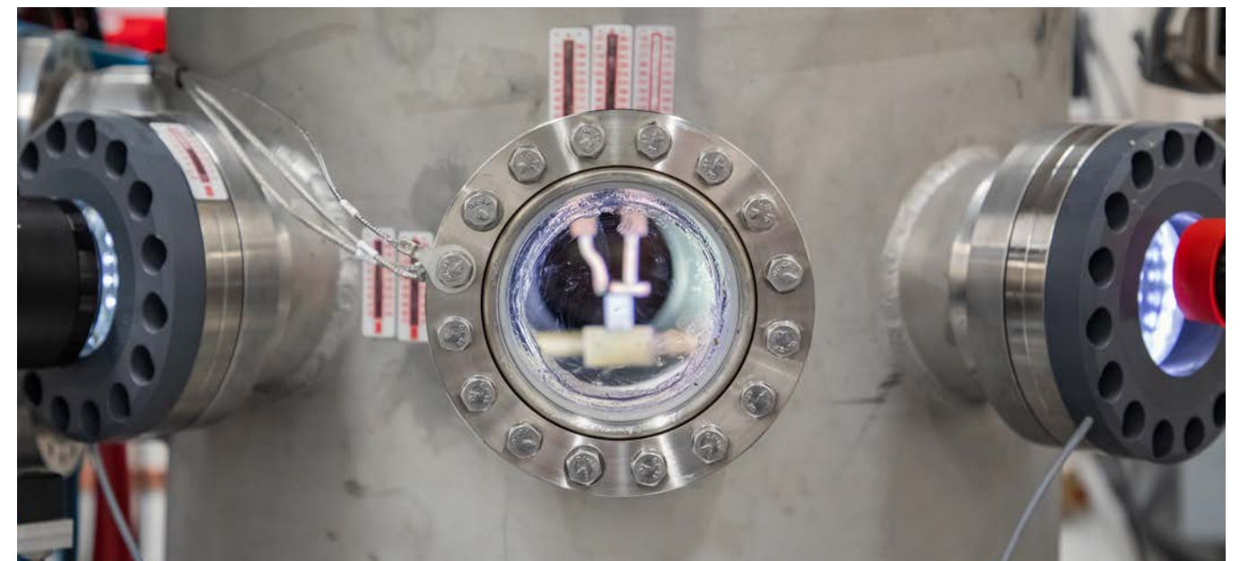
HIVE - The Heat by Induction to Verify Extremes facility is a unique test platform that forms part of a suite of testing rigs and facilities.
