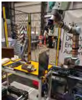
b) Robotic arm mounted on an actuated rail to deploy sensor rig.
