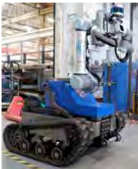
a) Robotic arm mounted on a mobile robot used to deploy sensor rig.
