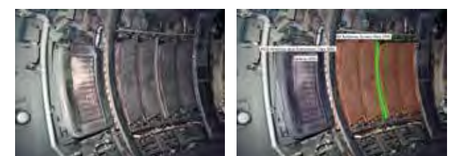
Figure 1: Detection of Mushroom Tiles in JET: a) original raw image and b) prediction results after analysis with trained deep learning model.
