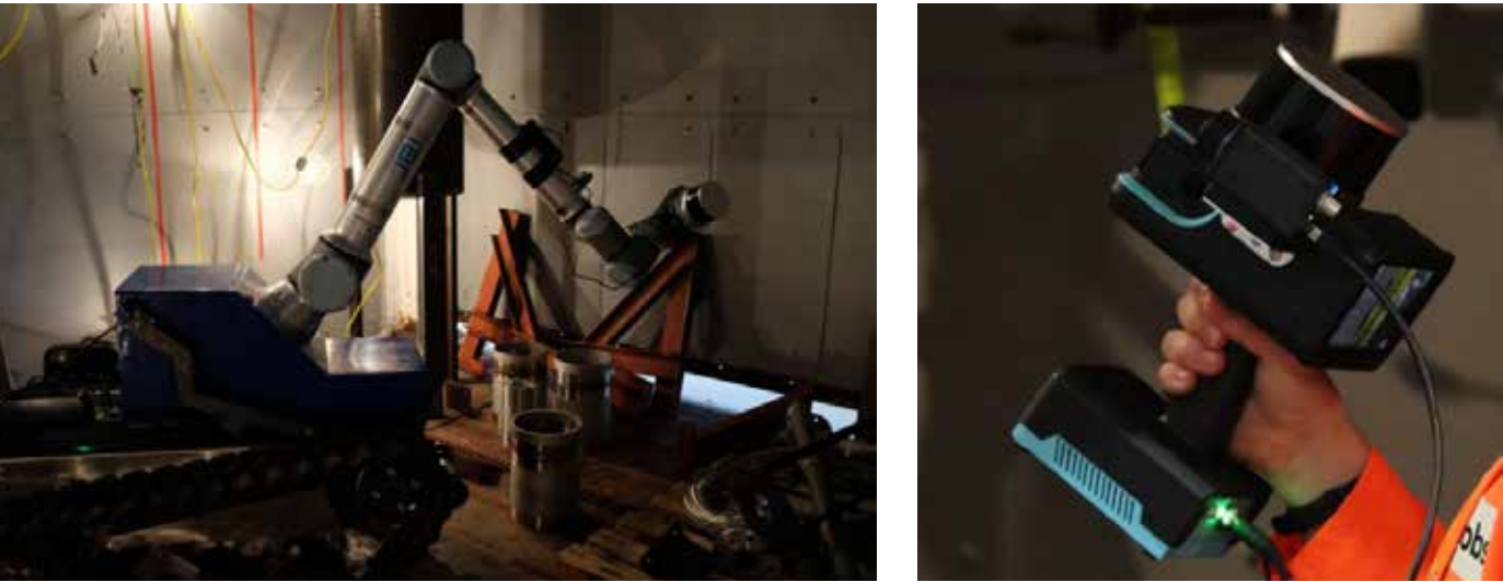
a) Frontier scanner mounted on a mobile robotic platform. b) Hand-held version of the scanner.
