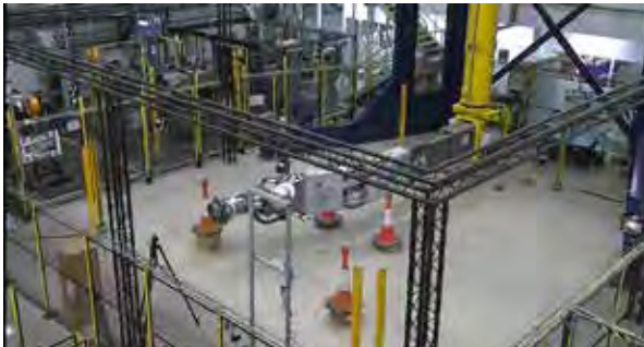
Figure 1 - Path planning and physical obstacle avoidance tests using TARM at UKAEA RACE.
