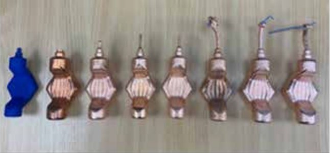
Picture from the Ultima Forma components formed during trailing and optimisation phase of the Electroforming-Enabled HIP for Complex Component Manufacturing
