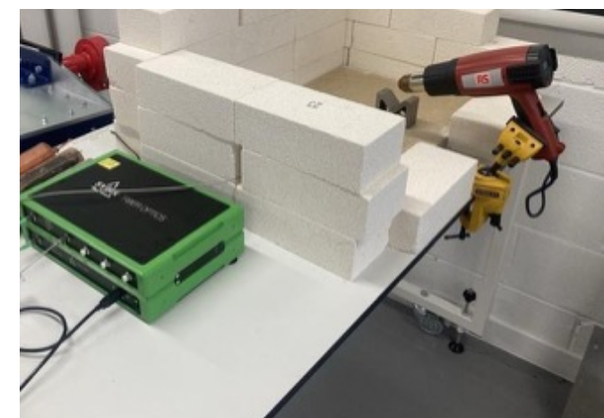
Figure 12: Experimental setup for the pipe heating experiment, including an interrogator to process the readings from the fibre sensors.
