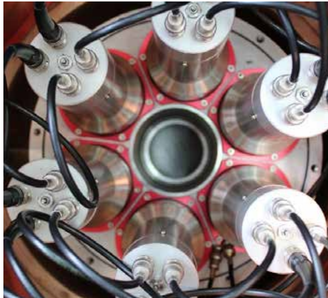
Figure 39: The Mirion Broad Energy Germanium (BEGe) detector used in this work, with the physical Compton suppression system surrounding the main HPGe crystal. The MLCSA produced the same suppression effects as this bespoke (expensive) system, but with no cost.
