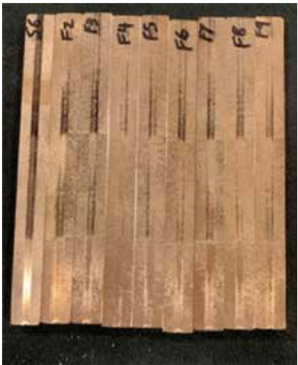
Figure 23: Samples of Phase 2b, with REBCO tape embedded into the copper substrate before electrical testing.
