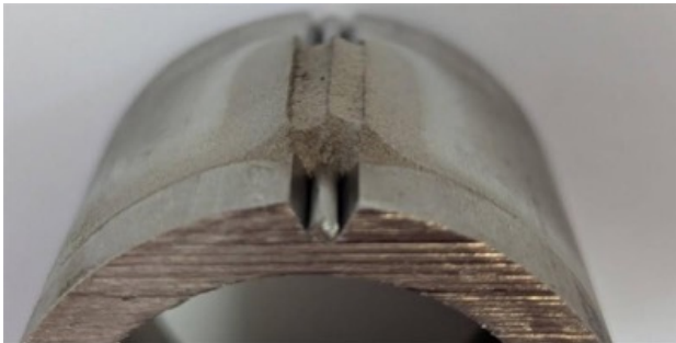
Figure 14: Successfully embedded steel rod by cold spray deposition in the initial manufacturing trials.
