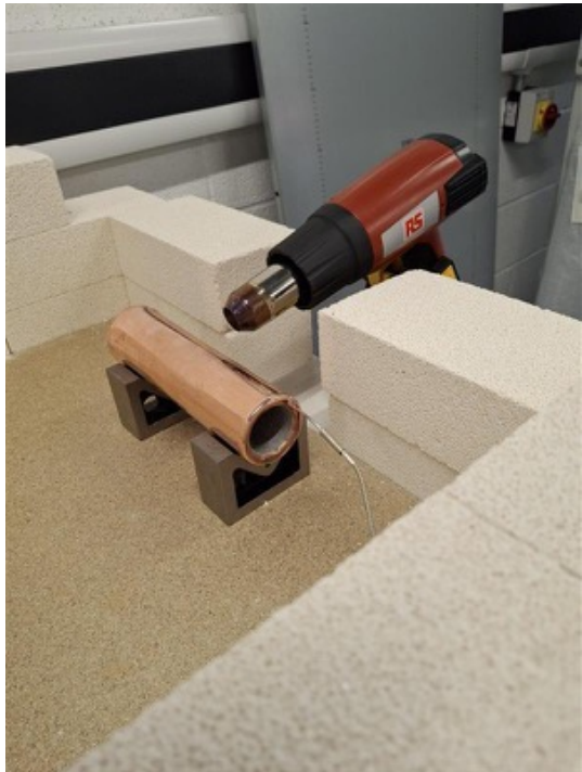
Figure 13: Copper electroplated pipe with embedded sensor ready for heating.
